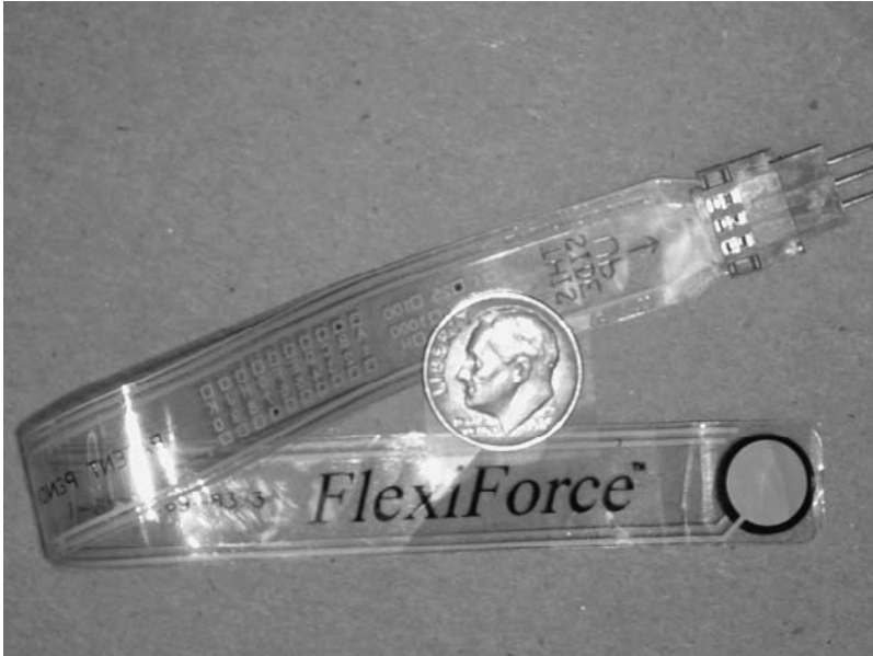
FIGURE 7.7 A FlexiForce force-sensing resistor. (Courtesy of Tekscan, Inc., http://www.tekscan.com/flexiforce.html .)
